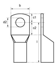
Image 4-1 Dimensions of the cable lugs
