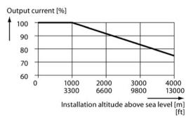
Image 6-4 Derating of the output current in accordance with the installation altitude with frame size GX
