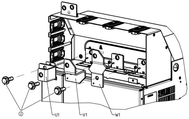
Image 4-6 Installing the mounting kit, step 2
