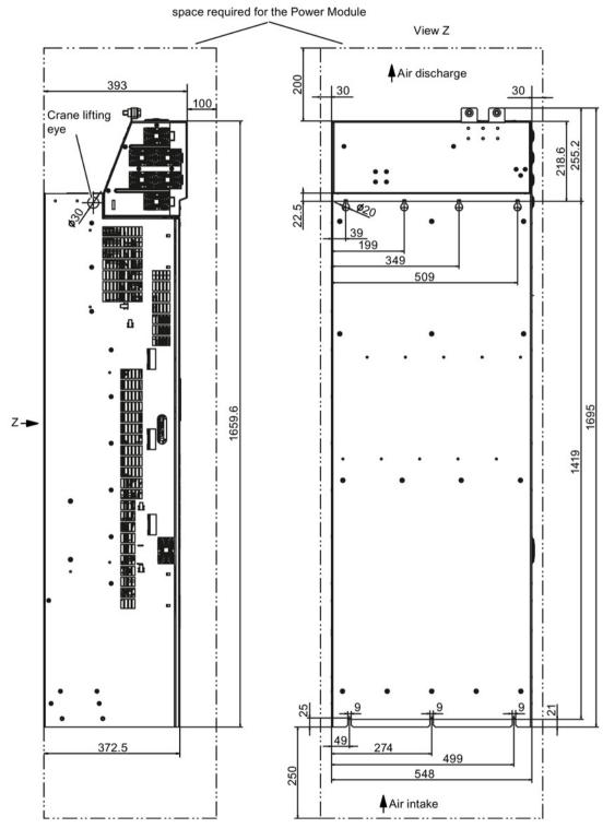
Image 3-5 Dimension drawing of PM330 frame size HX, view from the side, view from the rear
