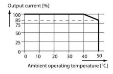
Image 6-3 Derating factor of the output current as a function of the operating temperature
