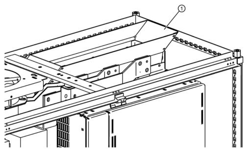
Image 3-1 Example of an air discharge duct
