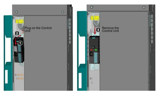
Image 3-7 Mounting and removing the Control Unit
