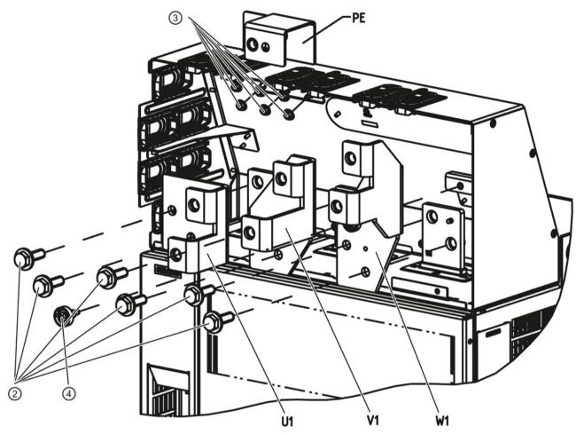
Image 4-10 Installing the mounting kit, step 2
