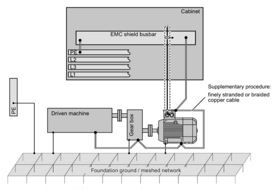
Image 4-14 Additional high-frequency bonding of the drive system
