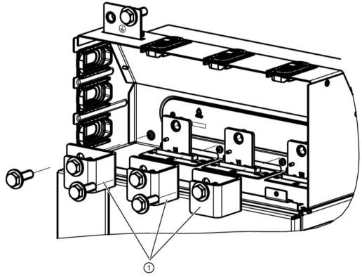
Image 4-5 Installing the mounting kit, step 1
