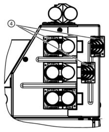
Image 4-8 Installing the mounting kit, step 4
