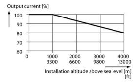
Image 6-5 Derating of the output current as a function of the installation altitudes for frame sizes HX and JX
