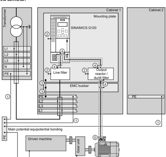
Therefore, connect the protective ground conductor and the cable shield to the motor and to the converter.
