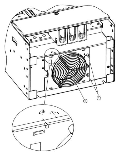
Image 5-3 Fan removal for frame size GX, view from below
