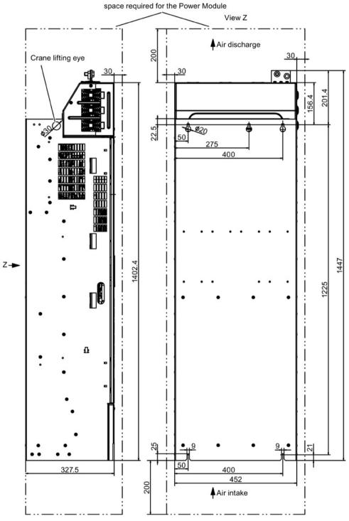
Image 3-4 Dimension drawing of PM330 frame size GX, view from the side, view from the rear
