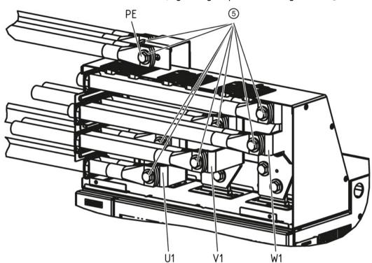
3. Final state with mounted installation set, tightening torque for the fixing screws ⑤: 50 Nm
