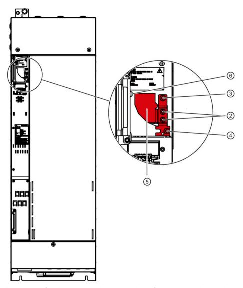
Image 4-4 Opening the connection to the basic interference suppression module
