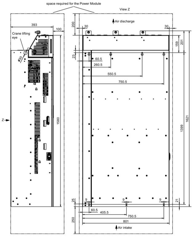
Image 3-6 Dimension drawing of PM330 frame size JX, view from the side, view from the rear
