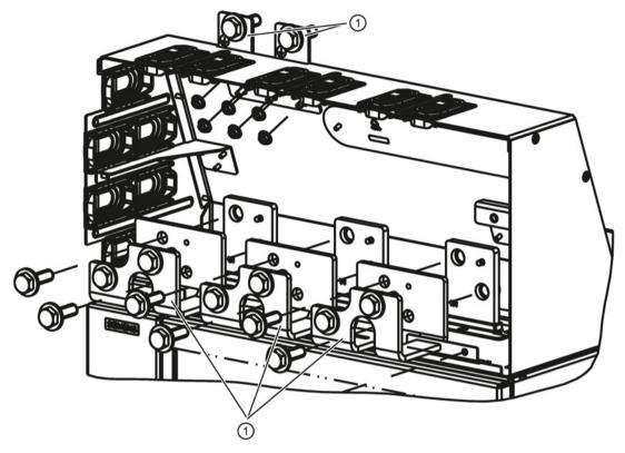
Image 4-9 Installing the mounting kit, step 1
